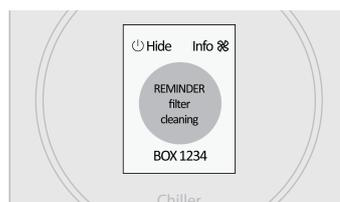
The filter cleaning reminder is displayed when the fan has been running for a certain amount of hours (default is 8000 h).
